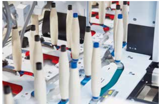
Fig. 2: Multilink systems with Multiflot can process up to four different material feeds.
