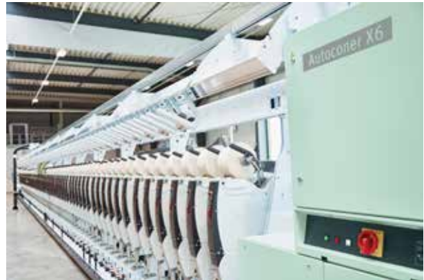
Fig. 1: The Autoconer X6 is the final quality assurance in the ring & compact-spinning process
