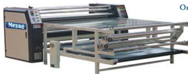
Heat Transfer Roll to Roll and Pieces With Different Size and Speed Up To 3 m/min
